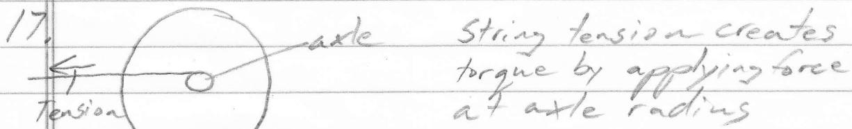
String tension creates torque by applying force at axle radius
