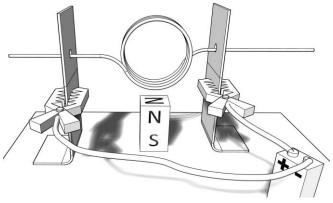
4. In the diagram below a magnet is being pushed into a stationary conducting ring. In what direction is the induced current flowing through the near side of the ring?
