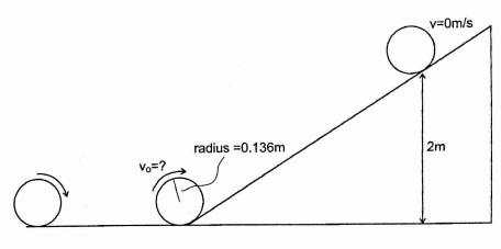
What was the disc's linear velocity when it first reached the bottom of the ramp (just before it began to ascend)?
