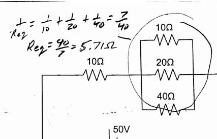
B. Calculate the total current flowing through this circuit.
