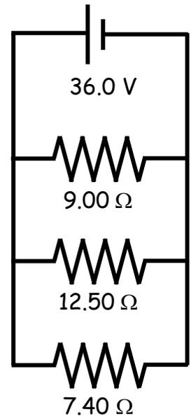
6. A. Calculate the total equivalent resistance of this circuit.
