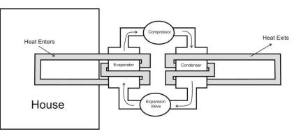
evaporator takes energy from its environment, cooling everything around it, including the grey pipes. In the summer, the homeowner would want these cooling pipes inside the house. In the condenser, the refrigerant condenses, and in order to do that, the refrigerant needs to lose heat. As the refrigerant condenses, it release its heat to its environment, heating up everything around it – including the grey pipes that wrap around it. During the summer, these hot pipes need to be outside the house.
