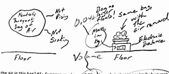
How hot is the air in this bag? #1: Suppose you have a 0.25m bag of air that is neutrally buoyant in the surrounding air. It is hovering. The density of the surrounding air is 1.2kg/m³. You remove all of the air from the bag, and you measure the mass that remains. That mass is 0.04kg.
