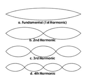
occur at integer multiples of the fundamental frequency. For example, if the fundamental frequency is 10Hz, the 2nd harmonic would have a frequency of 20Hz; the 3rd harmonic would be 30Hz; the 4th harmonic = 40Hz. For wavelength, this relationship is inverted. The wavelength of the  $2^{nd}$  harmonic is ½ the fundamental wavelength. The  $3^{rd}$  harmonic's wavelength is 1/3 the fundamental wavelength
