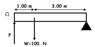
II. Find the location of the fulcrum so that the bar balances. In case A), assume the bar has negligible mass. In cases B) and C), the location of the center of mass is again designated by the downward arrow and the W.
